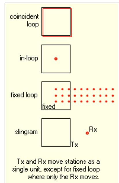
**Figure 2 - Loop geometries.**
