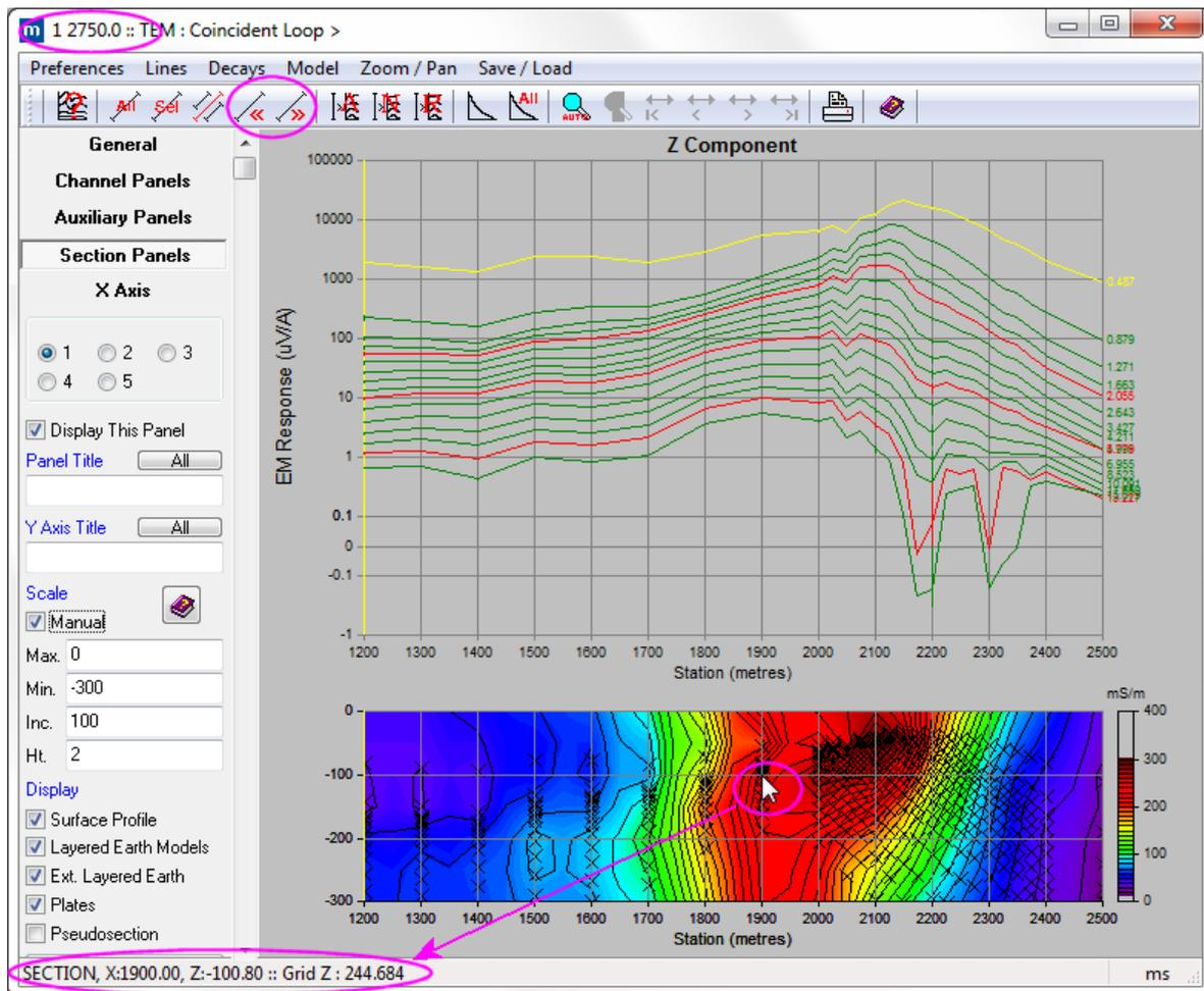
Figure 11 - Profile Window display of Emax conductivity data.
