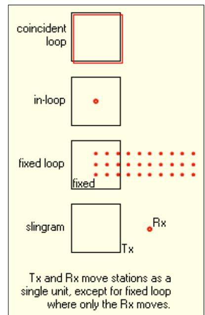
**Figure 2 - Loop geometries.**
