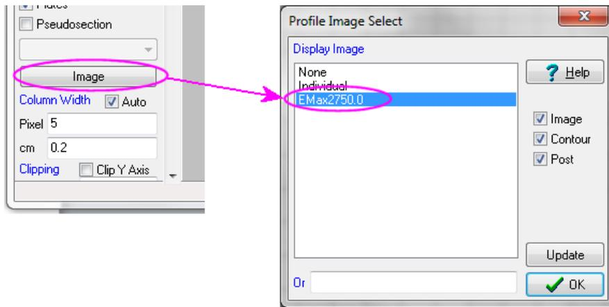
Figure 10 Select image to display in the section panel.
