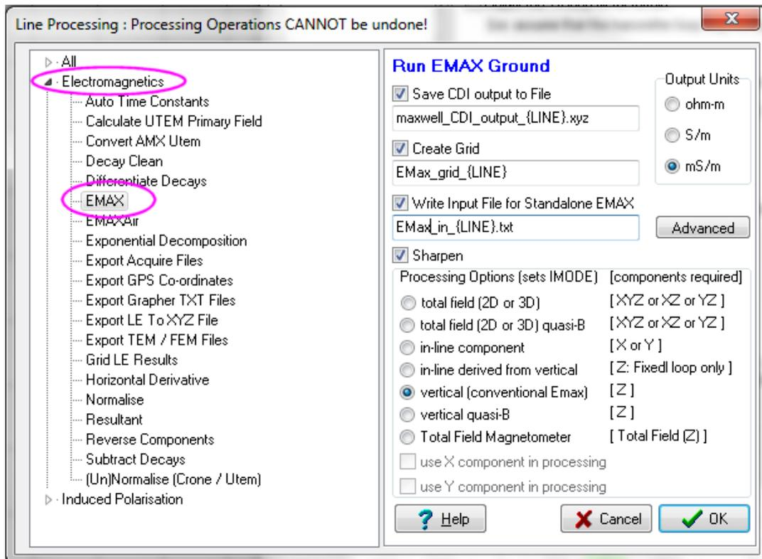
Figure 6 - Selecting basic options for Emax.
